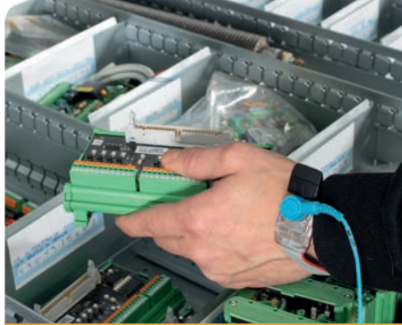
ESD protection system
